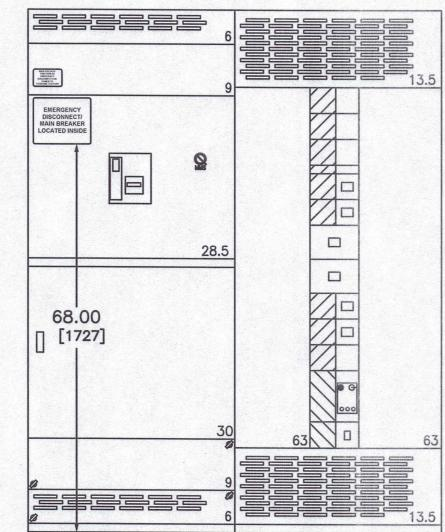
B EMERGENCY DISCONNECT SIGN HEIGHT DETAIL D-4 SCALE: N.T.S.
