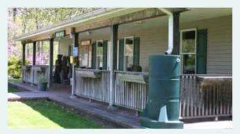
Rain barrels allow rain water from a building's roof to be collected on-site and slowly discharged after the rain storm to reduce the peak flow of stormwater in nearby streams that can occur during a storm.]
