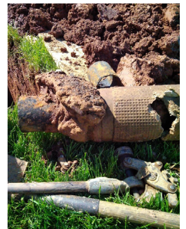
A failed Transition: the different pipe types being encased in concrete as a simple method of joining.
